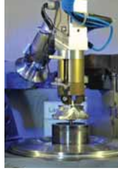
Forged-milled compressor wheel production
